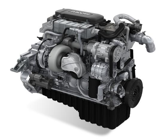
The 6.7 litre Euro 6 PACCAR PX-7 engine uses ultra-modern common rail technology, a turbo with variable geometry and advanced controls for maximum efficiency. In order to comply with the strict Euro 6 emissions requirements, it features exhaust gas recirculation, together with SCR technology and an active soot filter.
